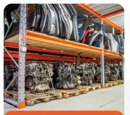
A designated area separate from the workshop is set aside to store new and displaced parts. Body parts are stored in racking system to help identification and protection against damage.
